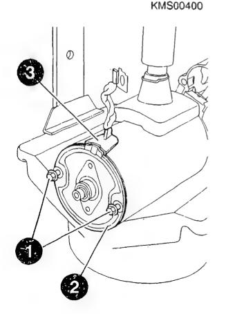
Assembling commutator end shield
